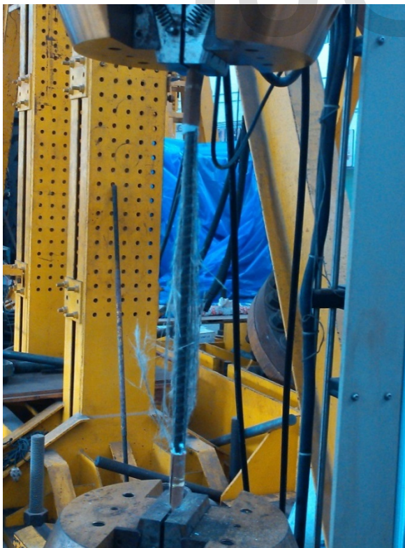
Fig. 2. Simple tension test on BFRP bar with failure at the middle region
