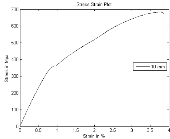
Fig. 3. Stress strain plot of the BFRP bar
